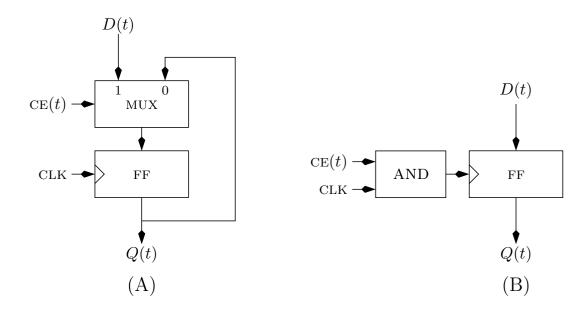
Question: Compute the parameters of the clock-enabled flip-flop depicted in part (A) in terms of the parameters of the edge-triggered flip-flop and the MUX.
