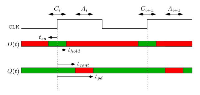
If the input D(t) is stable during the critical segments  $\{C_i\}_i$ , then the output Q(t) is stable in between the instability segments  $\{A_i\}_i$ .
