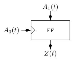
■ the signal  $A_0(t)$  is input as a clock to the flip-flop, but  $A_0(t)$  is not a clock.
