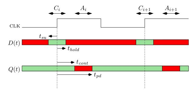
$$-t_{su} < t_{hold} < t_{cont} < t_{pd} \implies C_i \cap A_i = \emptyset.$$
