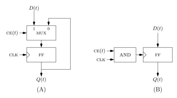
Question: Compute the parameters of the clock-enabled flip-flop depicted in part (A) in terms of the parameters of the edge-triggered flip-flop and the мих.
