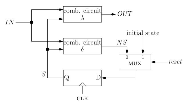
**Remark:** *NS* may not be logical during reset. Implementation of MUX must output initial-state if reset = 1. Implementation based on drivers has this property, while implementation based on combinational gates may not have this property. **Functionality of Synchronous Circuits: canonic form**
