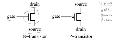
Inputs: gate & source Output: drain
