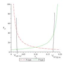
Figure:  $R_{sd}$  as a function of  $V_g$ .
