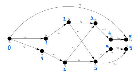
**Algorithm 2** longest-path-lengths (V, E) - An algorithm for computing the lengths of longest paths in a DAG. Returns a delay function d(v).
